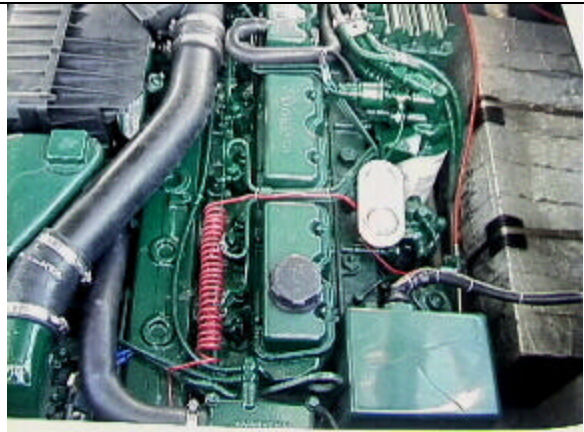
View of the port engine. Front 2 fuel injectors were leaking a small amount of diesel fuel. Silver manual temperature and pressure gauge has moisture behind the lens and gauge can't be read. Note secured rectangular water tank on the right side of photo.
