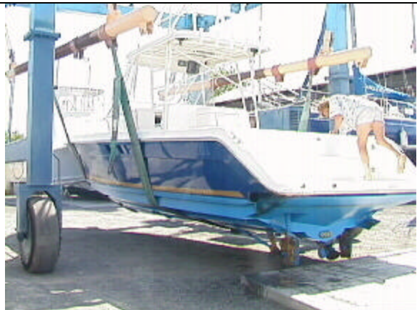
Port view of stern and side of boat being hauled at Oasis Marina. Note placement of slings. Note underwater running gear; drive shafts, struts, propellers, rudders, exhaust ports, trim tabs.
