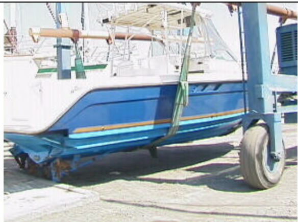
Starboard view of stern and side of boat being hauled at Oasis Marina. Note placement of slings, natural ventilation for engines.
