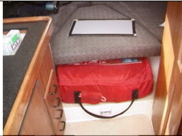
Eight (8) person life raft in the main cabin underneath the forward V berth.
